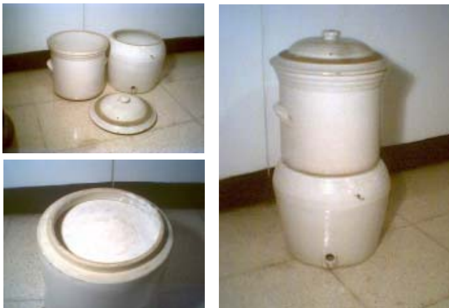
Figure 2.3: 100-Year Old Disk Filter from Spain
