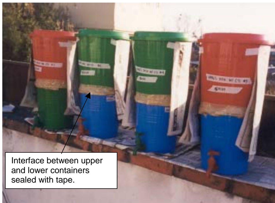
Figure 3.3: Laboratory Setup – Filter Systems Ready for Testing
