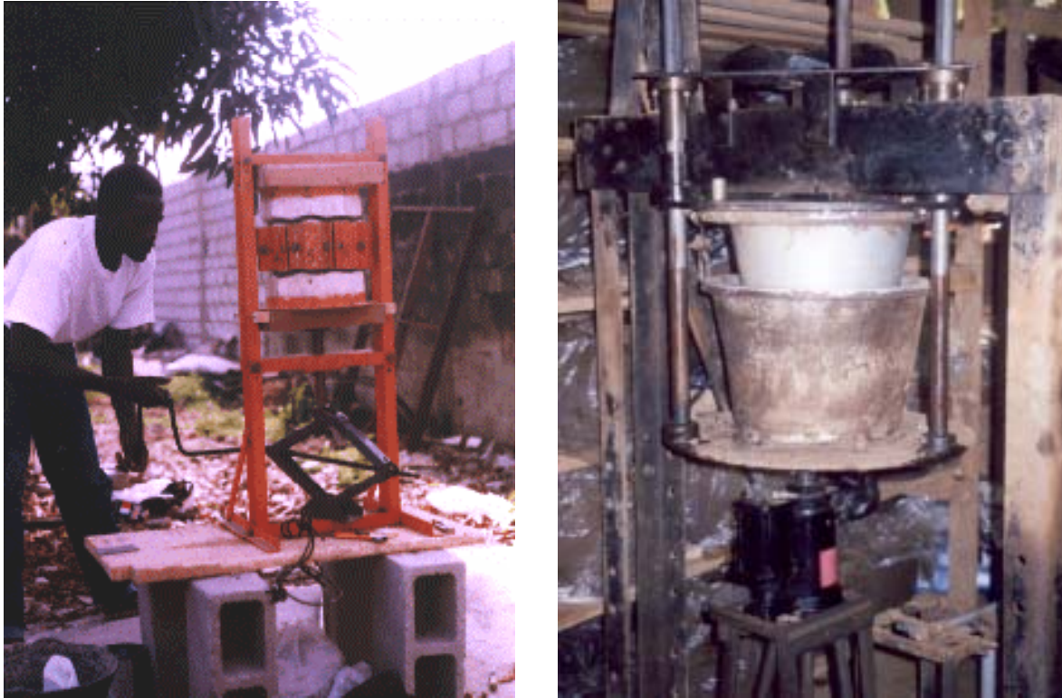
Figure 4.6: Example Filter Presses: Metal Frame and Car Jack (left), Hydraulic Jack System used by Potters for Peace (right).
