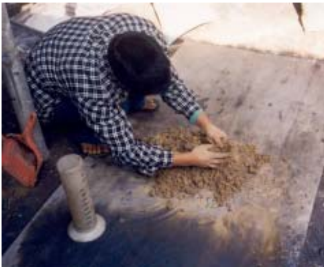
Figure 4.5: Worker Preparing a Mixture of Clay, Grog, and Water Madhyapur Clay Crafts, Thimi, Nepal. January 2003.
